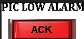
If the PIC value is below its limit, fix it and acknowledge the alarm.
