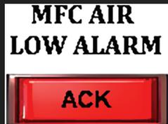
If the MFC air value goes below its limit, the alarm is stored. Correct the issue and acknowledge the alarm.
