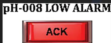
If the pH value drops below its limit, an alarm appears. Fix the pH, then acknowledge the alarm.
