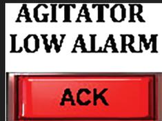
If the agitator speed goes below its limit, the alarm is triggered. Correct it and acknowledge.
