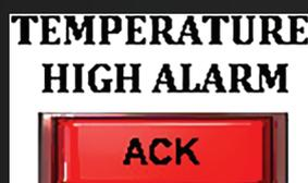
If the temperature exceeds its high limit, resolve it and acknowledge the alarm.
