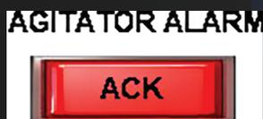
If the MCB trips or a cable is disconnected, an alarm is triggered. Fix the issue, then acknowledge it.
