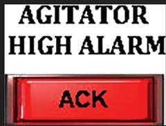
If the agitator speed goes above its limit, fix it, then acknowledge the alarm.
