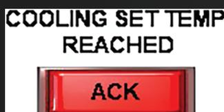
If the cooling set temperature is reached, the alarm is stored on the home page. Acknowledge it.
