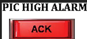
If the PIC value exceeds its high limit, resolve it, then acknowledge the alarm.
