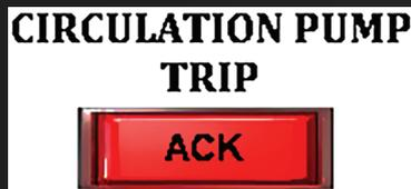
If the OLR trips, an alarm is triggered. Release the OLR button and then acknowledge the alarm.
