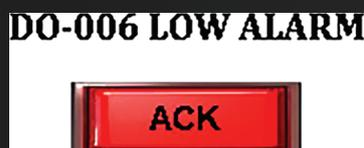
If the emergency button is pressed, an alarm will appear. Release the button, then acknowledge the alarm.
