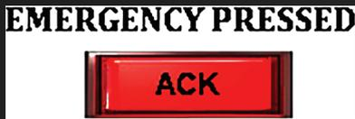
If the emergency button is pressed, an alarm will appear. Release the button, then acknowledge the alarm.
