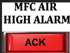
If the MFC air value goes above its limit, acknowledge the alarm after fixing the problem.
